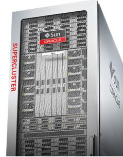
Four 5.1 GHz SPARC CPUs 256 hardware threads per CPU socket 64 MB L3 Cache 16 TB RAM 8 NVMe SSD for DB Storage + 12 Disks 40 G Infiniband 4 Quad 10G Ethernet
